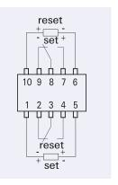
Latching, 2 coils reset condition
