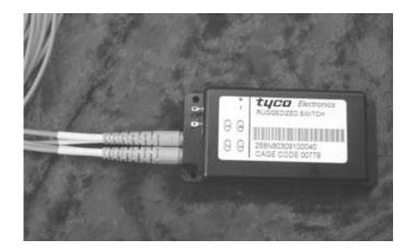
Tyco Electronics' "Ruggedized" Refractive Plate Switch is a multimode optical switch that is capable of withstanding a 200 G shock with a duration of >8ms without interruption of the signal path.
