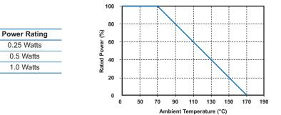
For resistors operated in ambient temperatures above 70°C, power rating must be derated in accordance with this curve.
