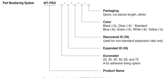
Example of standard product, MT-PBX72-100-X-6IN Example of non-standard product with adhesive lining, MT-PBX55A-120-080-X-SP
