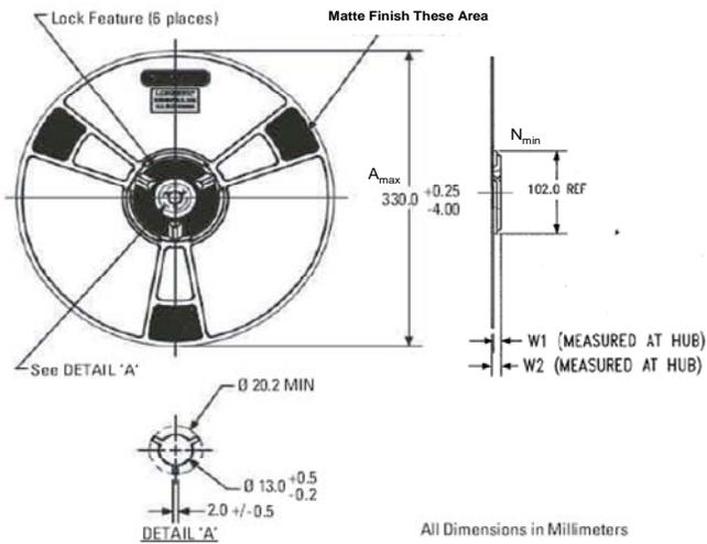
**Taped Component Dimensions for PolyZen Devices**
