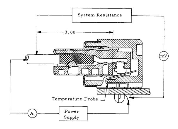
Voltage drop due to the 3" equivalent wire length is to be removed from all readings.
