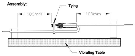
The variation in frequency is done by logarithmic scanning of one octave per minute. No micro cut-off longer than 1  $\mu$ s must appear during the test.
