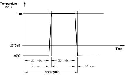
*Requirement*: The difference between the contact resistance value after conditioning and the initial contact resistance shall be less than 4 mOhms. However, this contact resistance shall never be greater than 6 mOhms.
