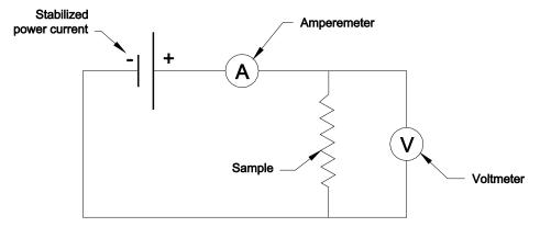
The measurements shall be made after thermal stabilization.
