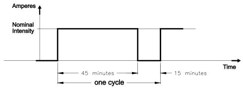
Nominal intensity = 7A x the cross-sectional area of a strand multiplied by the number of strands measured  $\pm 0.01$  mm.
