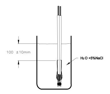
The transition time between the chamber and the bath does not exceed 30 seconds.
