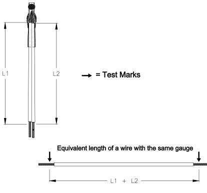
Re = the resistance of the specimen==> Ue = the voltage drop of the specimenRf = the resistance of an equivalent length of wire ==> Uf = the voltage drop of an<br/>equivalent wireRc = the contact resistance==> Uc = the drop due to the connection<br/>==> Ue - UfRcUc = Re - R==> Ue - Uf
