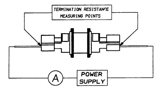
TERMINATION RESISTANCE MAY BE MEASURED OUTBOARD OF THE POINTS SHOWN. THE BULK RESISTANCE MUST THEN BE SUBTRACTED.
