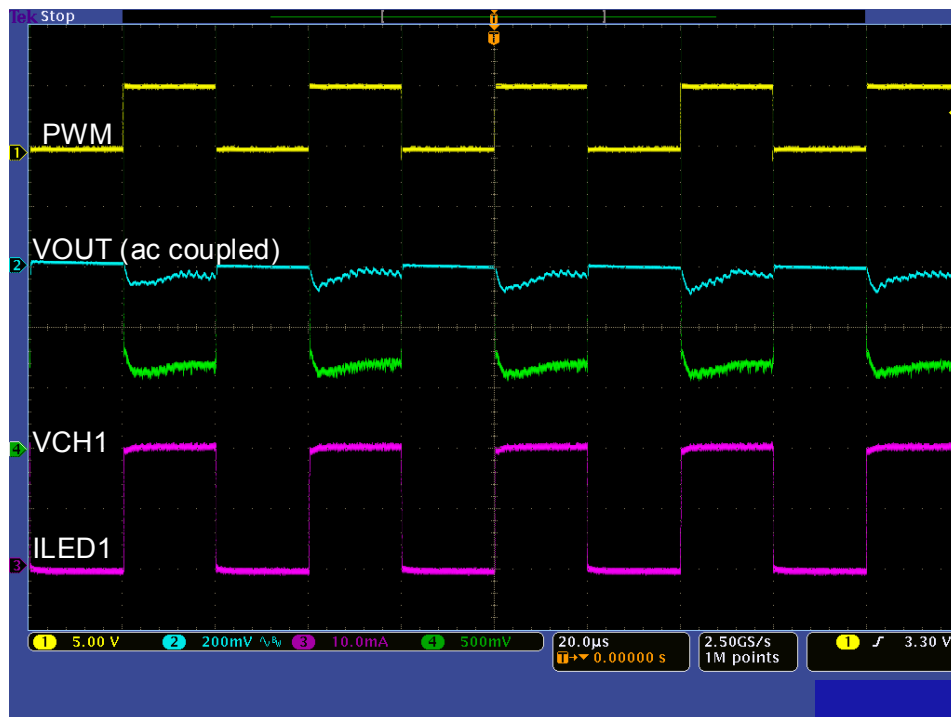
Figure 8. Typical Operating Waveforms (FPWM=25kHz, 50% duty)
