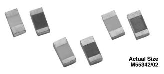
Thin Film Mil chip resistors feature all sputtered wraparound termination for excellent adhesion and dimensional uniformity. They are ideal in applications requiring stringent performance requirements. Established reliability is assured through 100 % screening and extensive environmental lot testing. Wafer is sawed producing exact dimensions and clean, straight edges.
