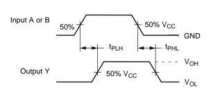
Figure 4. Switching Waveforms
