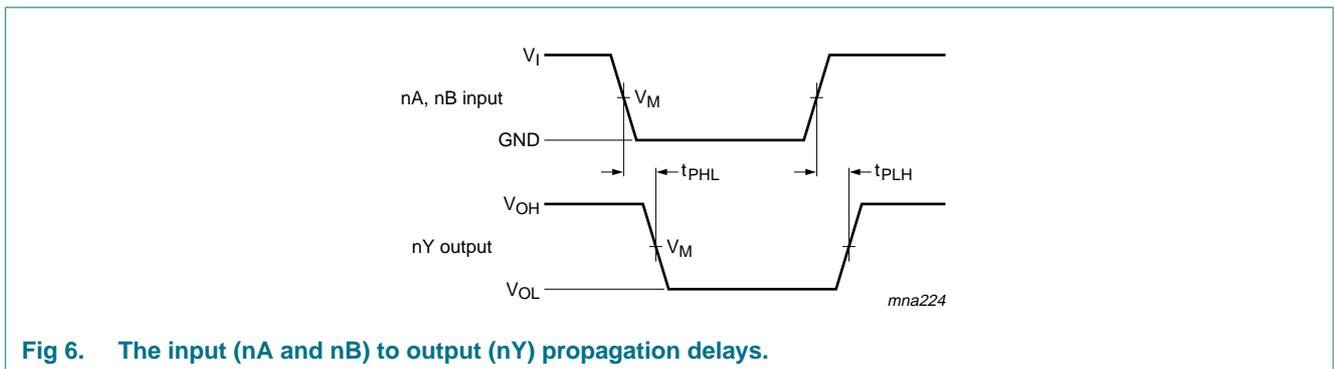
**Fig 6. The input (nA and nB) to output (nY) propagation delays.**
