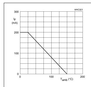
Device mounted on an FR4 printed-circuit board.
