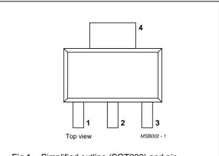
Fig.1 Simplified outline (SOT223) and pin configuration.
