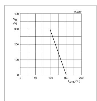
Fig.7 Maximum permissible continuous reverse voltage as a function of ambient temperature.
