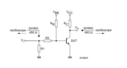
$$\begin{split} V_i = 5 \; V; \; T = 500 \; \mu s; \; t_p = 10 \; \mu s; \; t_r = t_f \leq 3 \; ns. \\ R1 = 56 \; \Omega; \; R2 = 2.5 \; k\Omega; \; R_B = 3.9 \; k\Omega; \; R_C = 270 \; \Omega. \end{split}$$
