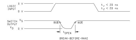
FIGURE 4. Timing diagram.
