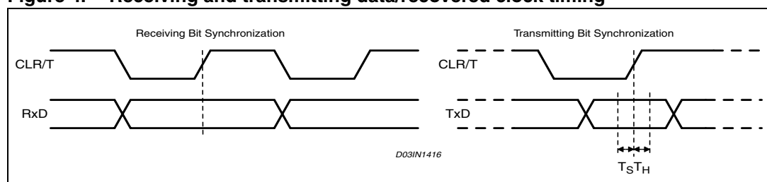
Figure 4. Receiving and transmitting data/recovered clock timing
