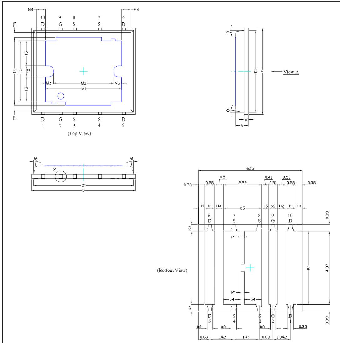
Figure 10. Recommended PAD layout
