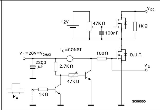
**Figure 4. Test circuit for inductive load switching and diode recovery times**
