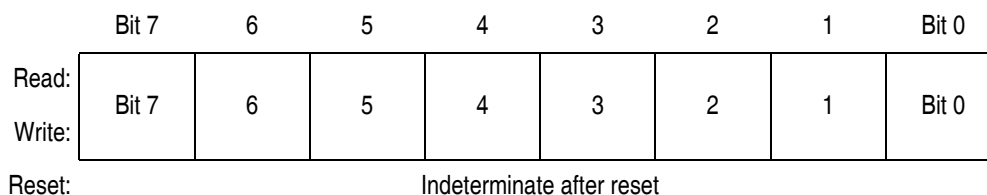
Figure 11-15. TIMA Channel 0 Register Low (TACH0L)
