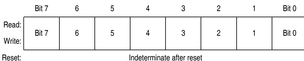
Figure 10-13. TIM Channel 0 Register Low (TCH0L)
