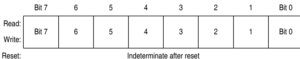
Figure 10-15. TIM Channel 1 Register Low (TCH1L)
