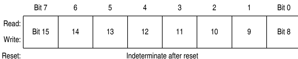
Figure 10-14. TIM Channel 1 Register High (TCH1H)
