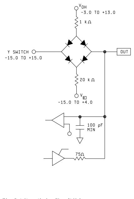
1. VOH and VOL will be adjusted to meet load conditions of table I.
