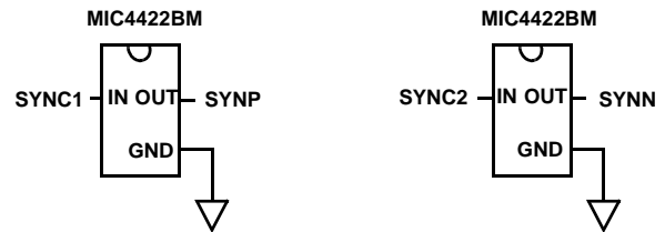
FIGURE 22B. NON-INVERTING DRIVERS
