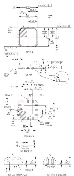
L20.6x6B 20 LEAD QUAD FLAT NO-LEAD PLASTIC PACKAGE (COMPLIANT TO JEDEC MO-220VJJB ISSUE C)
