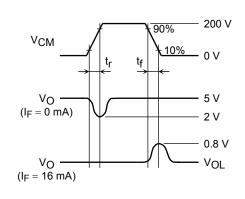
Note: CM<sub>H</sub>: The maximum tolerable rate of rise of the common mode voltage to ensure the output will remain in the high output state (i.e.,  $V_O > 2.0 V$ ). Measured in volts per microsecond (V/µs).
