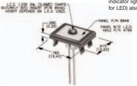
Above frames (part nos. 432XXXXXX) are also available with insert which accepts LED for indicator light assembly. Order insert separately from frame. Blank insert panel (without hole for LED) also available. **LED not included.**
