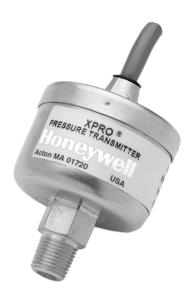
The XPRO industrial grade pressure transmitter provides instrument engineers and OEM designers with reliable and affordable measurements. The 4 mA to 20 mA output signal is well suited for long cable runs in electrically noisy environments.
