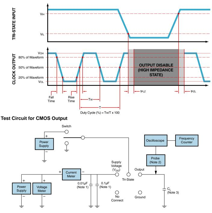
Note 1: An external  $0.1\mu$ F low frequency tantalum bypass capacitor in parallel with a  $0.01\mu$ F high frequency ceramic bypass capacitor close to the package ground and V<sub>DD</sub> pin is required.
