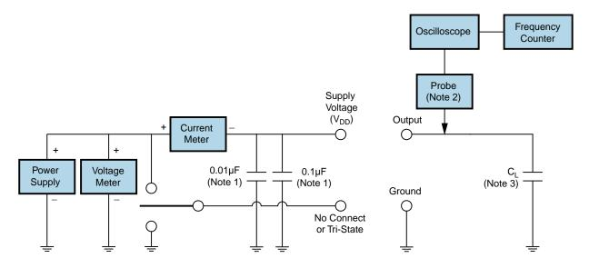
Note 1: An external  $0.1\mu F$  low frequency tantalum bypass capacitor in parallel with a  $0.01\mu F$  high frequency ceramic bypass capacitor close to the package ground and  $V_{DD}$  pin is required.
