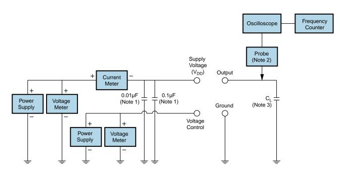
Note 1: An external 0.1µF low frequency tantalum bypass capacitor in parallel with a 0.01µF high frequency ceramic bypass capacitor close to the package ground and V<sub>DD</sub> pin is required.
