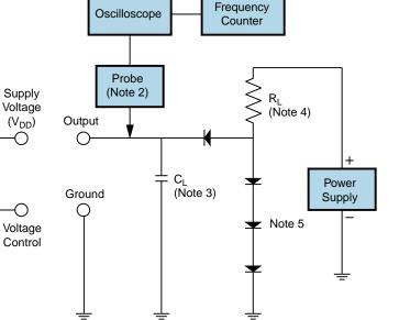
Note 1: An external  $0.1\mu F$  low frequency tantalum bypass capacitor in parallel with a  $0.01\mu F$  high frequency ceramic bypass capacitor close to the package ground and  $V_{DD}$  pin is required.
