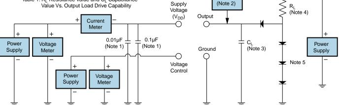
Note 1: An external 0.1µF low frequency tantalum bypass capacitor in parallel with a 0.01µF high frequency ceramic bypass capacitor close to the package ground and  $V_{\text{DD}}$  pin is required.
