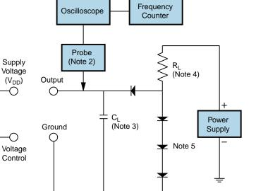
Note 1: An external  $0.1\mu\text{F}$  low frequency tantalum bypass capacitor in parallel with a  $0.01\mu\text{F}$  high frequency ceramic bypass capacitor close to the package ground and  $V_{DD}$  pin is required.
