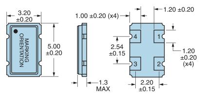
Note: Pin 1 Chamfer not shown.
