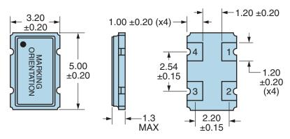
Note: Pin 1 Chamfer not shown.
