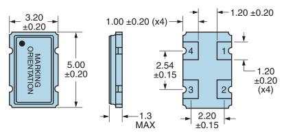
Note: Pin 1 Chamfer not shown.
