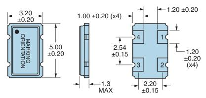
Note: Pin 1 Chamfer not shown.
