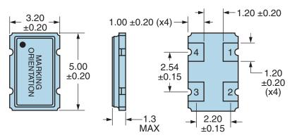
Note: Pin 1 Chamfer not shown.
