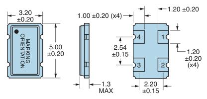
Note: Pin 1 Chamfer not shown.
