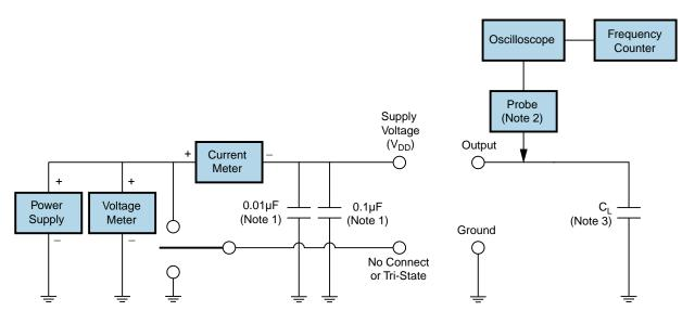
Note 1: An external  $0.1\mu F$  low frequency tantalum bypass capacitor in parallel with a  $0.01\mu F$  high frequency ceramic bypass capacitor close to the package ground and  $V_{DD}$  pin is required.
