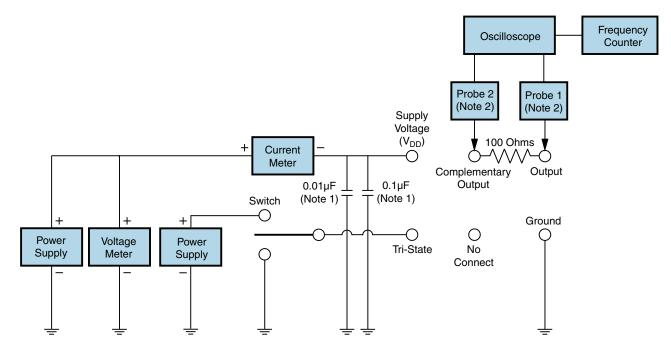
Note 1: An external 0.01µF ceramic bypass capacitor in parallel with a 0.1µF high frequency ceramic bypass capacitor close (less than 2mm) to the package ground and supply voltage pin is required.
