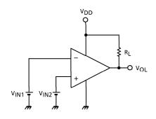
$V_{OL}$   $V_{IN1} = \frac{V_{DD}}{2} + 0.05V$   $V_{IN2} = \frac{V_{DD}}{2} - 0.05V$
