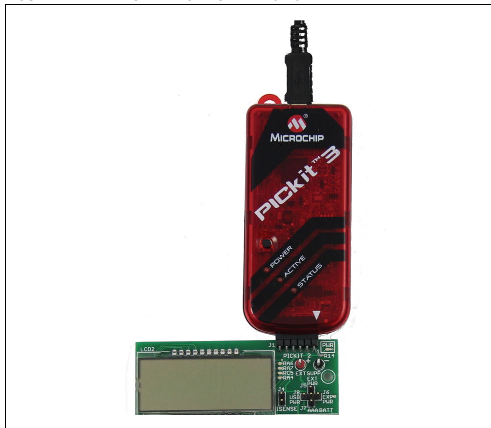
FIGURE 2-2: POWERING FROM PICKit™ 3
