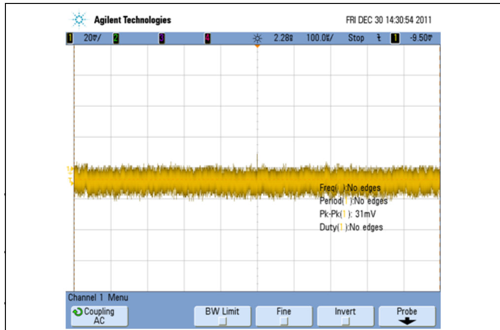
FIGURE 2-5: V_{OUT} Ripple of the Evaluation Board is less than 30 mV p-p using RC Snubber and R_{BOOST} (12V Input, 100 mA Load). Compare to Figures 2-3 and 2-4.
