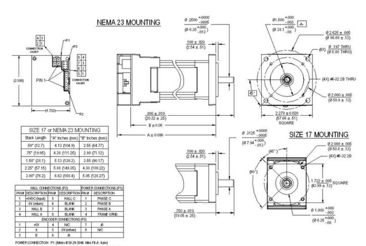
HALL CONNECTIONS P2: (Molex#70543-0007 C-Grid St. Connector 8 pin)
