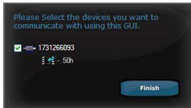
Figure 8 - ADP1043A address in the GUI
