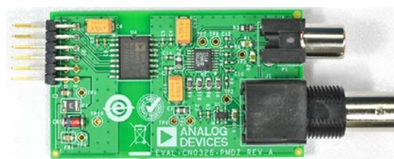
Figure 7. Photo of EVAL-CN0326-PMDZ Board
