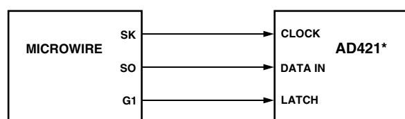
Figure 9. AD421 to MICROWIRE Interface
