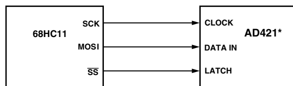
Figure 8. AD421 to 68HC11 Interface
