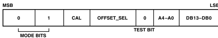
b. 24-Bit Input Serial Write Word (DAC Mode)
