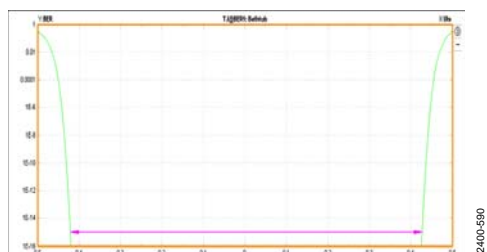
Figure 131. Bathtub, External 100 \Omega Terminations at 10 Gbps
