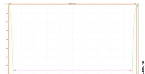
Figure 137. Bathtub, External 100 \Omega Terminations at 6 Gbps
